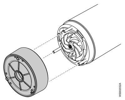
5. Mount the strainer and the screws. Tightening torque: 9.3 Nm (6.9 ft-lb)
