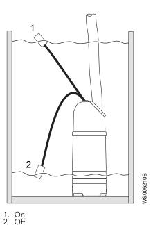
Figure 1: The functionality of the level regulator
