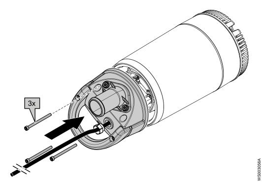
4. Tighten the cable entry.
