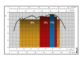
All the new Z6 series pumps offer a superior efficiency and therefore all points selected between 14 m³/h and 70 m3/h have always efficiency equal to or higher than 70% with a max efficiency of 77% within the overall Z6 range.
