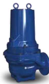
Lowara 1320 Vortex Maximum flow 54 l/s Maximum pressure 29 m Motor Rating 3.5 - 7.5 kW Outlet 80 - 100 mm Weight 140 - 156 kg
