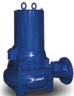
Lowara 1325 Non-clog Maximum flow 115 l/s Maximum pressure 63 m Motor Rating 9 - 18 kW Outlet 80 - 150 mm Weight 170 - 190 kg
