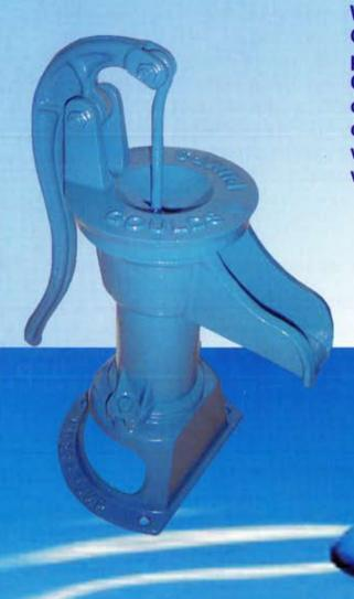
Working replica of the original 1848 Goulds heavy duty hand operated pitcher water pump with open spout. Capable of pumping water from cisterns or wells with levels up to 25 ft. (7.5 m) deep. Ideal use as intended for drawing water from wells or as decoration water features.
